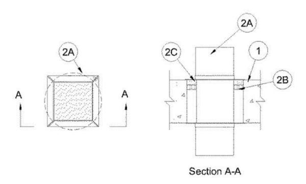
Floor or Wall Assembly — Min 2-1/2 in. ( 64 mm) thick reinforced lightweight or normal weight (100-150 pcf or 1600-2400 kg/m³) concrete. Wall may also be constructed of any UL Classified Concrete Blocks\*. Max diam of opening is 6 in. (152 mm) for square devices, 2-1/2 in. (64 mm) for 2 in. (51 mm) round devices and 4-1/2 in. (114 mm) for 4 in. (102 mm) round devices. When thickness of floor or wall assembly is less than 4-1/2 in. (114 mm), T Rating is 1/2 Hr.
