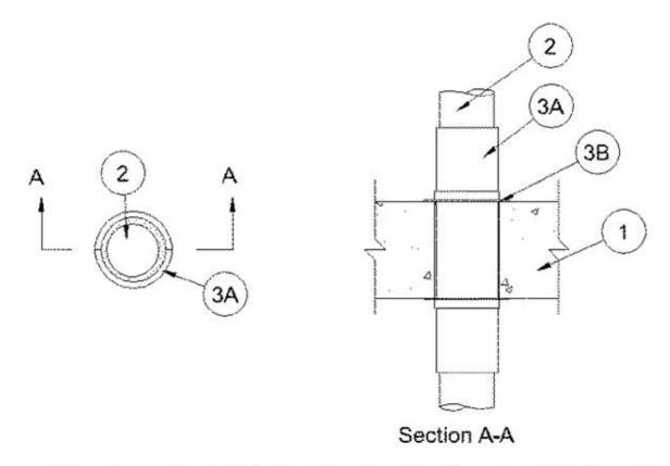
Floor or Wall Assembly — Min 2-1/2 in. ( 64 mm) thick reinforced lightweight or normal weight (100-150 pcf or 1600-2400 kg/m³) concrete. Wall may also be constructed of any UL Classified Concrete Blocks\*. Diam of opening shall be 2-1/2 in. (64 mm) or 3-1/2 in. ( 89 mm) for nom 2 and 3 in (51 and 76 mm) devices.
