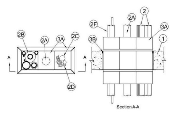
Floor or Wall Assembly — Min 2-1/2 in. ( 64 mm) thick reinforced lightweight or normal weight (100-150 pcf or 1600-2400 kg/m³) concrete. Wall may also be constructed of any UL Classified Concrete Blocks\*. Max area of opening is 56 1/4 in.² (363 cm²) with a max dimension of is 12 1/2 in. (318 mm) for square devices. Max diam of opening is 4-1/2 in. (114 mm) for round devices.
